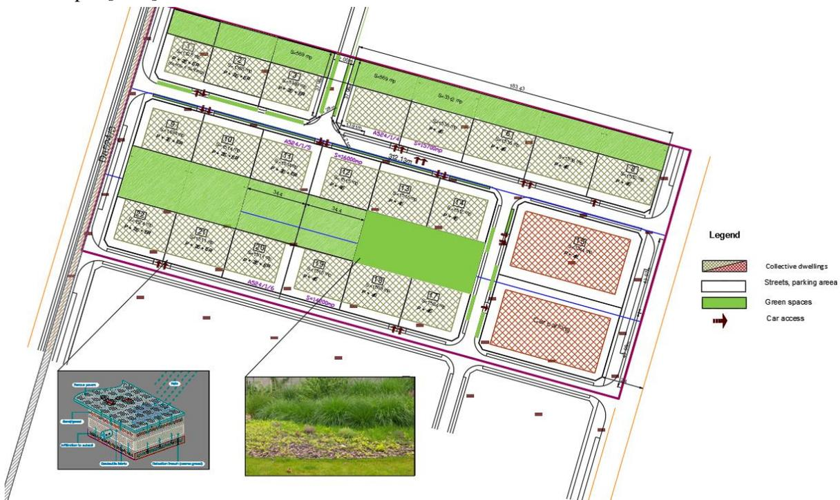
Fig. 3. Urban development proposal with bioretention basins and porous pavements [12]
